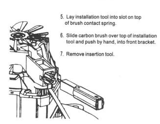
8. Using a rawhide mallet, gently tap carbon brush flush with bracket.
